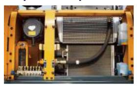
Open lateral structure makes maintenance convenient.
