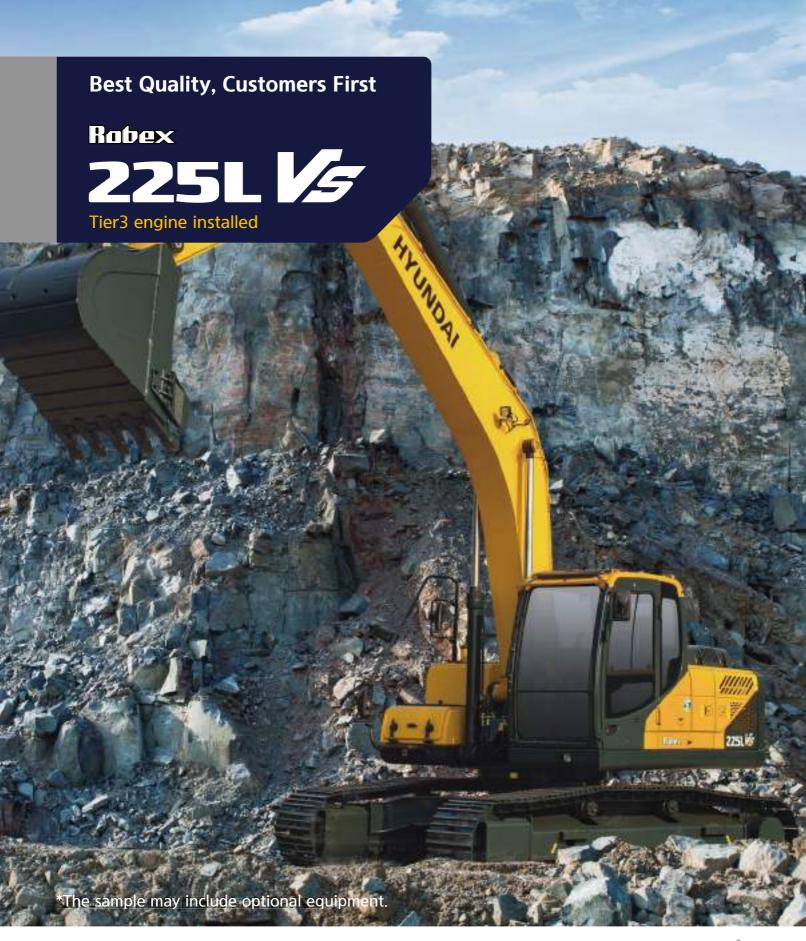
Net Power: 125kw(167HP)/1,900rpm | Operating weight: 22,570kg | Bucket capacity: 1.05m<sup>3</sup>
